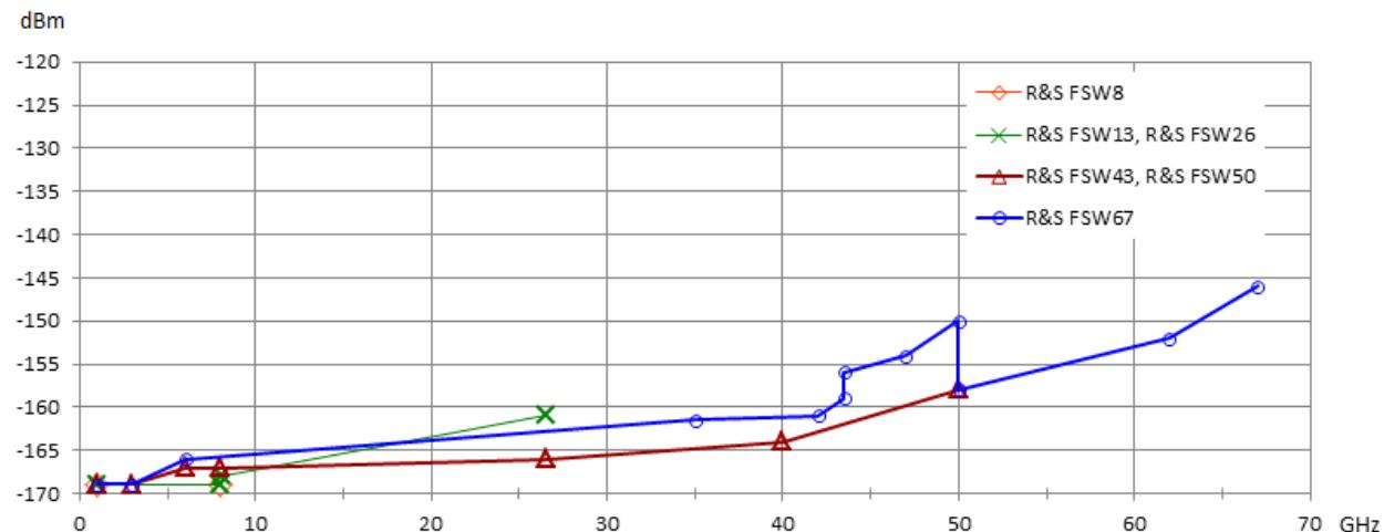
Typical displayed average noise level of the R&S®FSW models for  $f > 1$  GHz with R&S®FSW-B24<sup>7</sup> RF preamplifier option,
